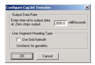
**Output Data Rate:** This is the interval, in milliseconds, that the output string is to be transmitted at. Enter 0 to inhibit output.
